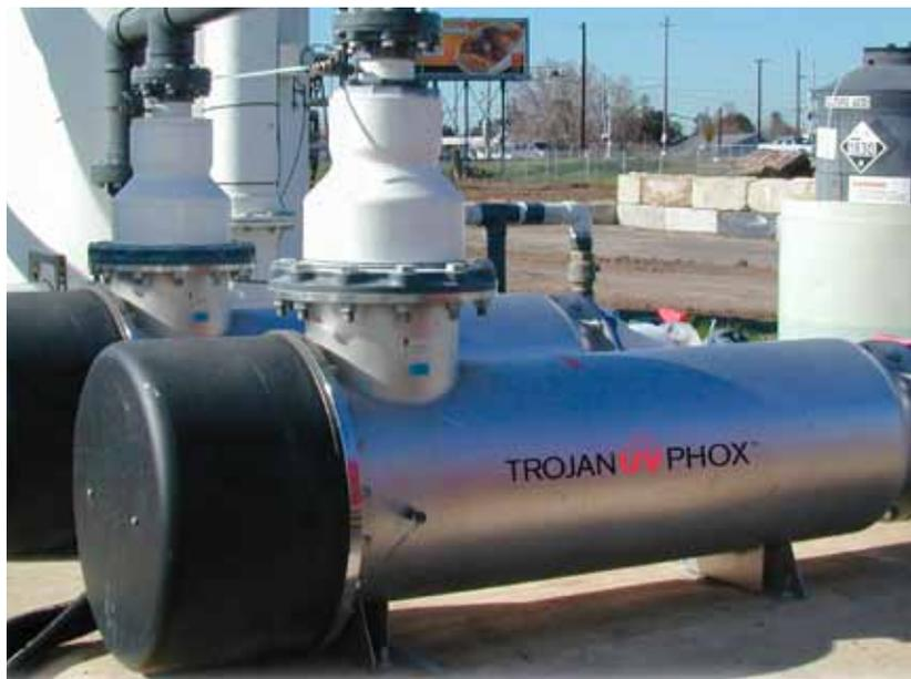
Figure 1. TrojanUVPhox™ system treating 1,4-dioxane
